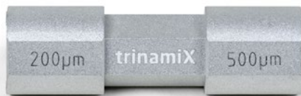
Figure 1: The Liquid Analysis Stamp. The left side provides a layer thickness of 200 \mu\text{m} , the right side a layer thickness of 500 \mu\text{m} as indicated on the stamp.
